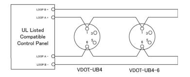
The VDOT-H3 or VDOT-H3(-H) detectors all have the three connections, and the terminals are configured as below.
